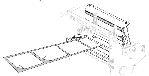
**10.** Remove the hook from the rewind spindle.
